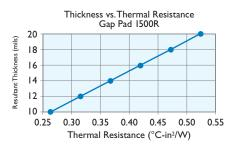
Thermally Conductive, Reinforced Gap Filling Material
